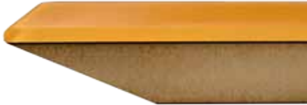
40620 1.25" reverse knife edge, KrystalCast Acrylic (.25" acrylic/ 1" subtop)
